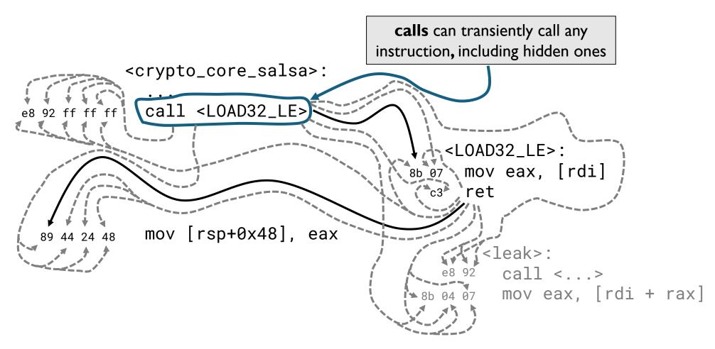
**Solution #I**: Use Intel ISA extensions to constrain speculative control-flow
